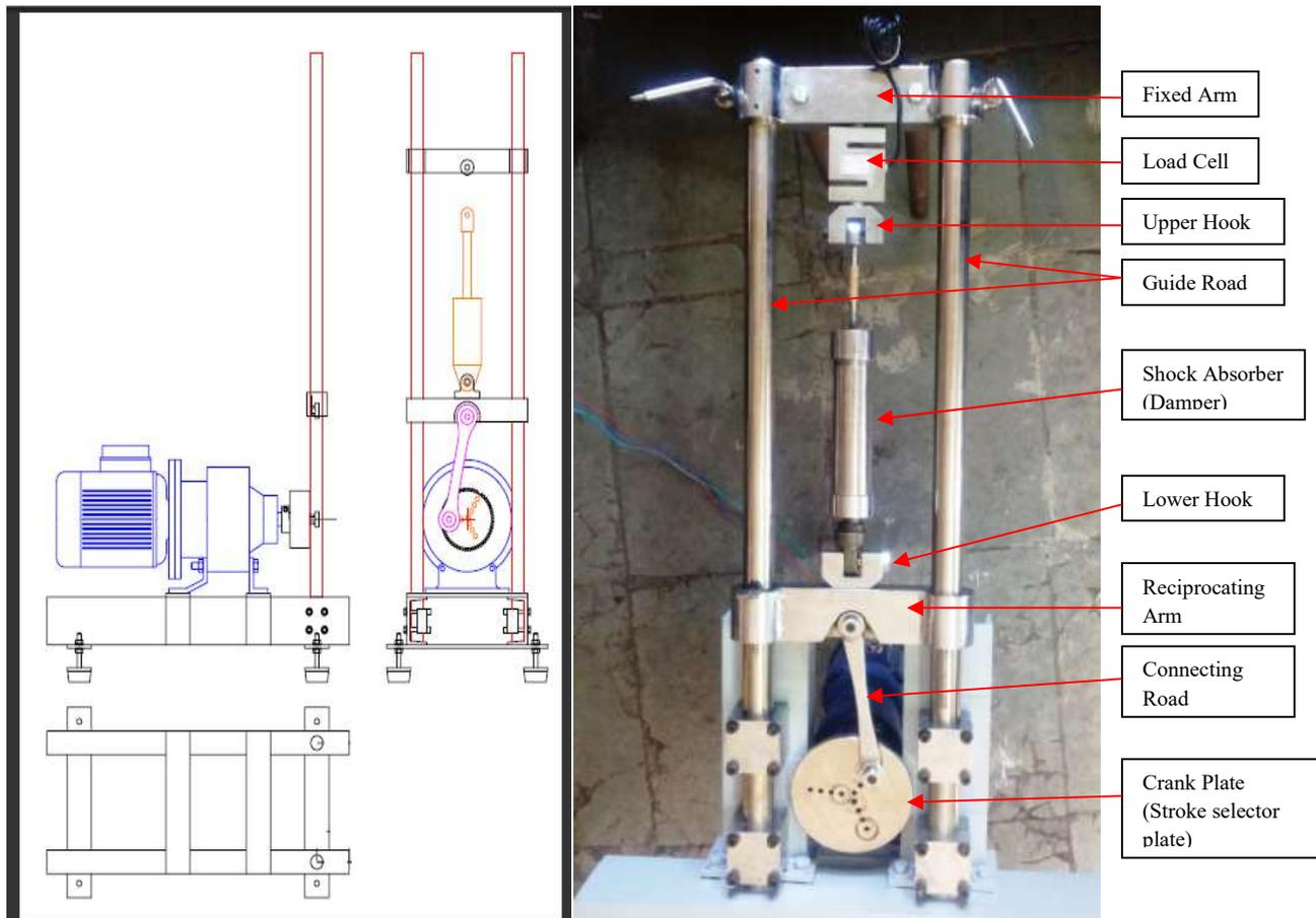
Figure 7. Shock absorber test rig
