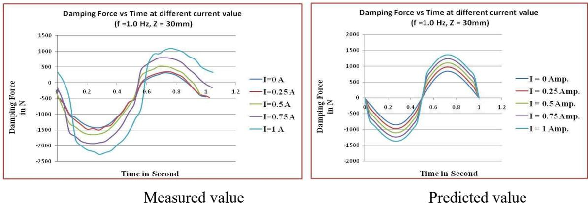
Figure 8-C: Force-Time relationships under 1.5 cm amplitude for different current values at  $f = 1$  Hz
