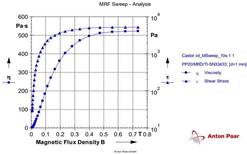
Figure 3. Relation between Magnetic flux density, Viscosity and Shear stress
