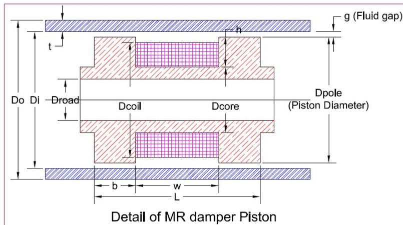
Figure 5. Details of proposed MR Damper Piston
