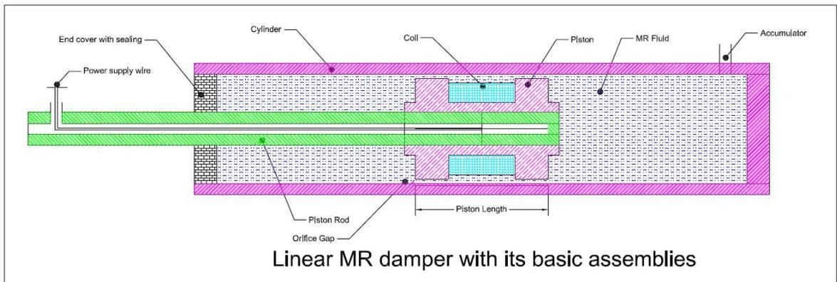
Figure 4. Basic assembly of proposed MR Damper
