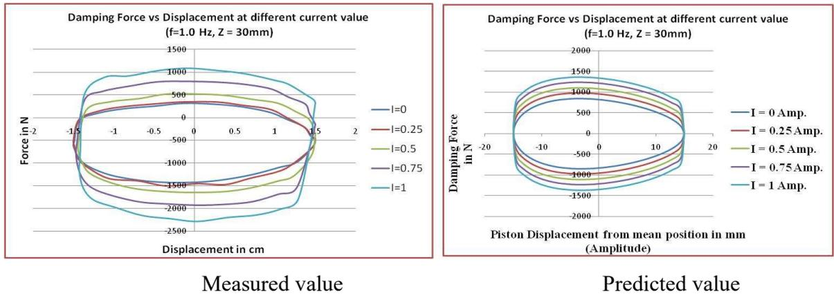
Figure 8-A: Force-displacement relationships under 1.5 cm amplitude for different current values at  $f = 1$  Hz
