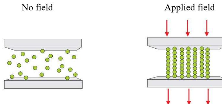
Figure 1: Chain-like structure formation in controllable fluids
