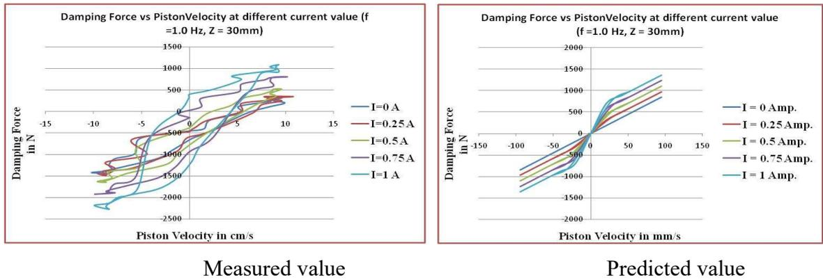
Figure 8-B: Force-velocity relationships under 1.5 cm amplitude for different current values at  $f=1$  Hz
