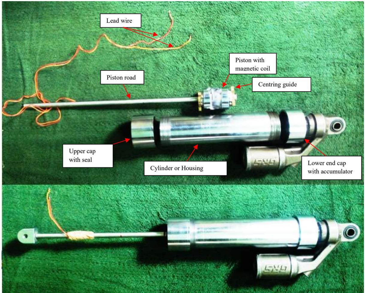
Figure 6. Real detail and assembly photo of predicted MR Damper
