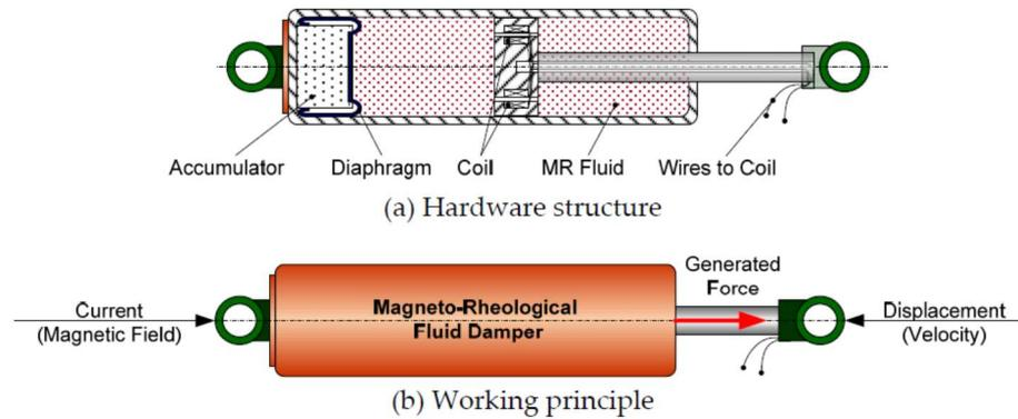
Figure 2. General configuration of a MR fluid damper.
